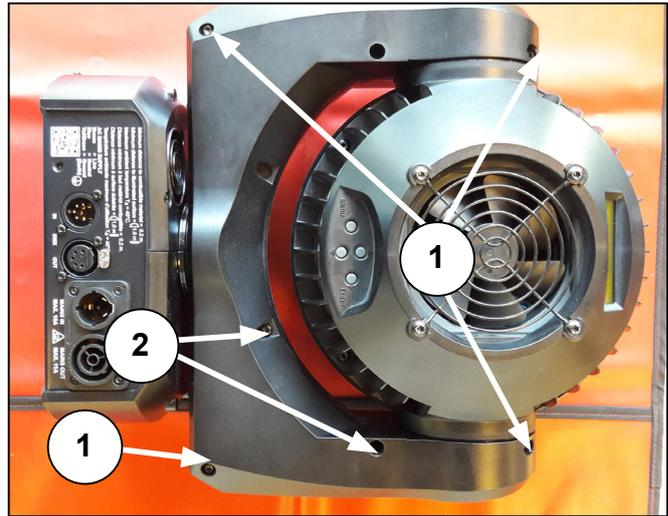
Figure 29: Removing the yoke covers
