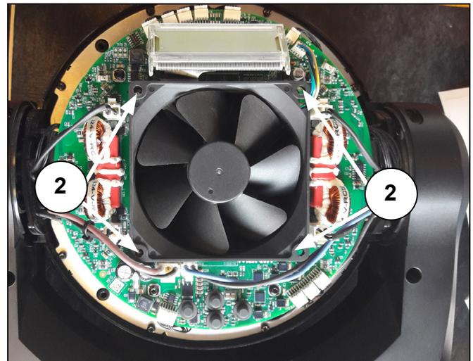
Figure 10: Removing the screws
