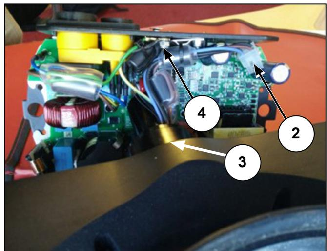
Figure 45: Disconnecting the connectors
