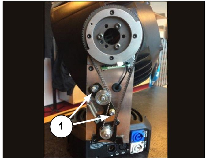
Figure 32: Adjusting the tilt timing belt
