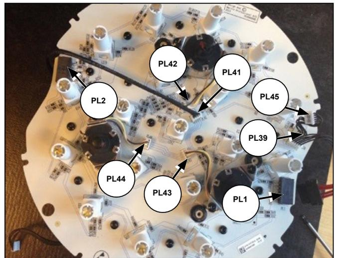
Figure 28: PCB connections
