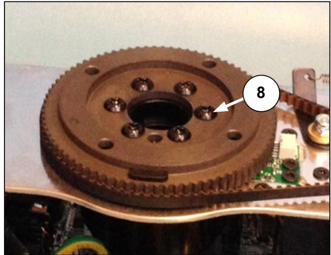
Figure 38: Removing the screws
