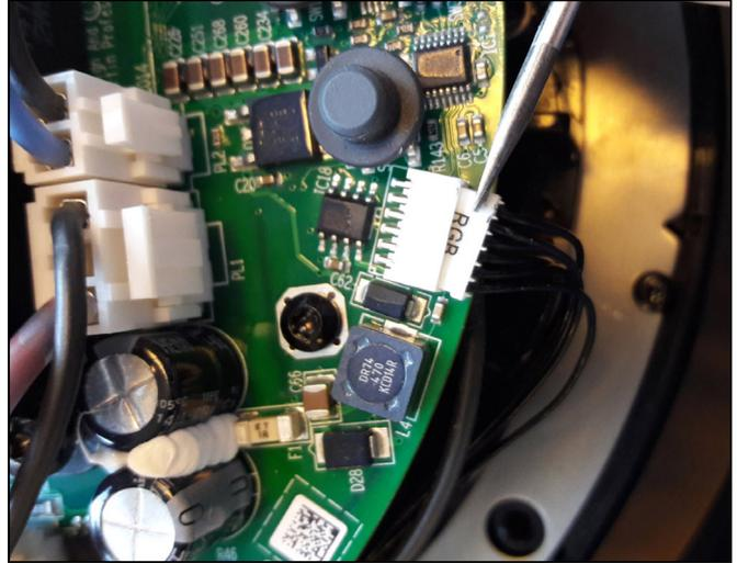
**Figure 7: Loosening the connectors**
