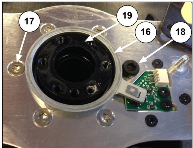
Figure 39: Replacing the gobo rotation belt
