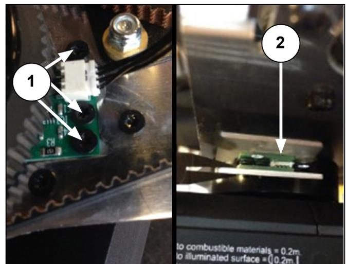
Figure 34: Replacing the pan reset sensor PCB
