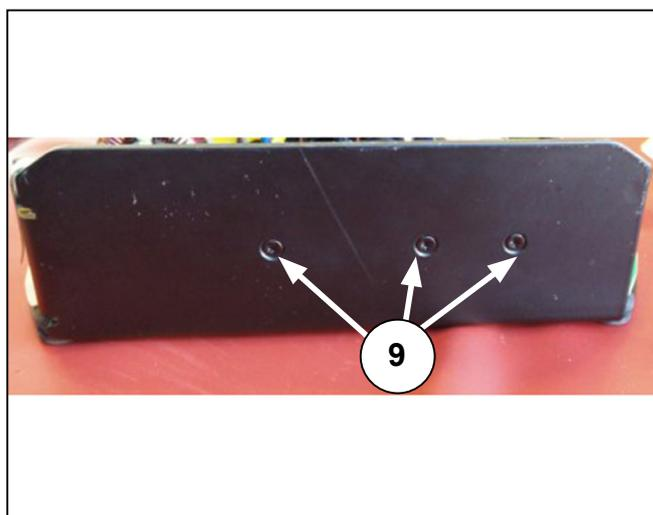
Figure 50: Screws holding the FET
