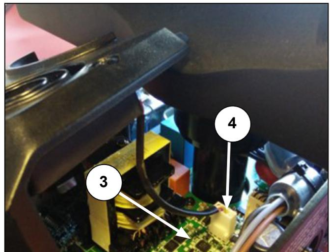
Figure 42: Connector for the fan wire
