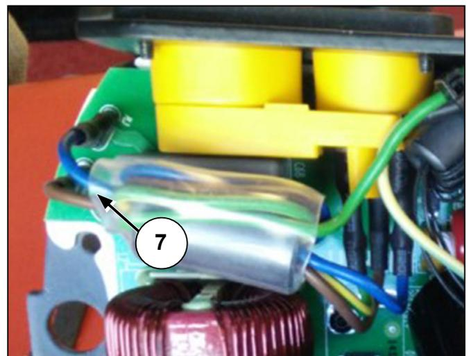
Figure 48: Mains wires
