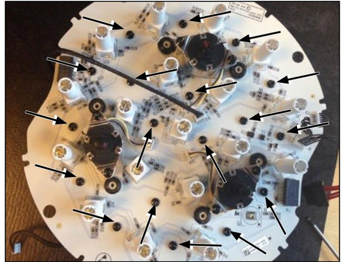
Figure 27: Replacing the primary pixel board
