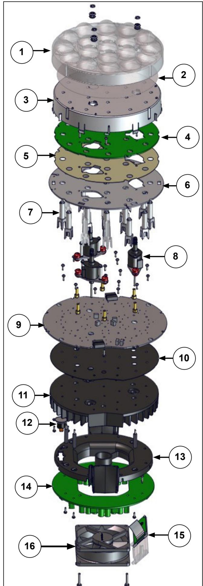
Figure 20: Exploded view of head assembly
