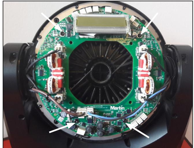
Figure 12: Removing the main PCB
