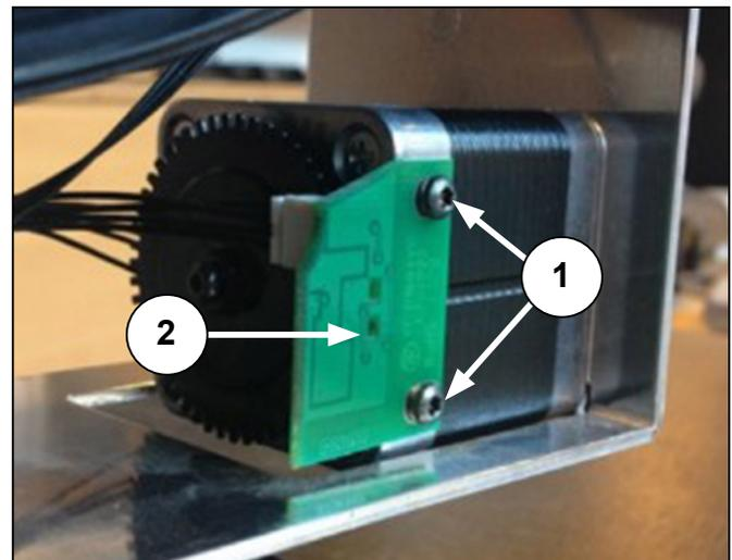
Figure 33: Replacing the tilt positioning sensor PCB
