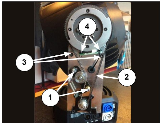
Figure 31: Tilt sensor and belt tensioner
