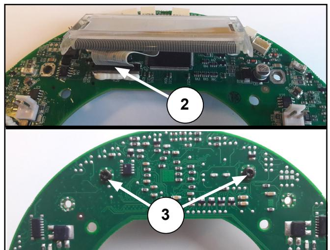
Figure 14: LCD display, ribbon cable and screws
