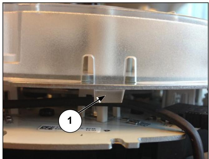
Figure 23: Diffuser plate taps
