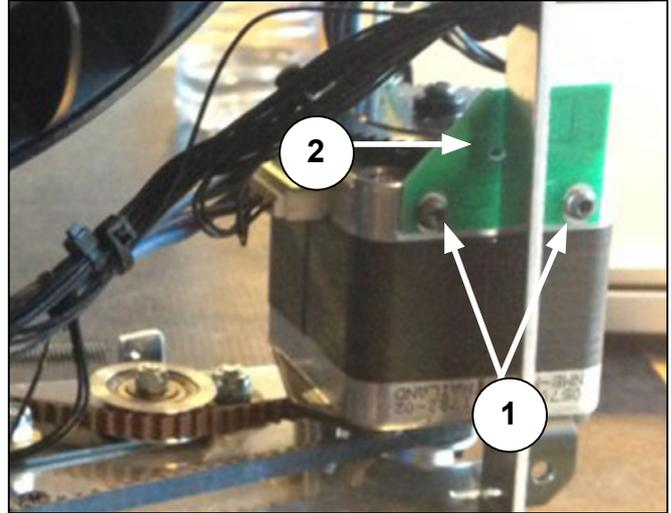
Figure 35: Replacing pan positioning sensor
