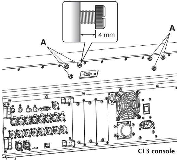
2. Hook holes 'B' of the MBCL mounting strap onto screws 'A' of the CL3/CL1.
