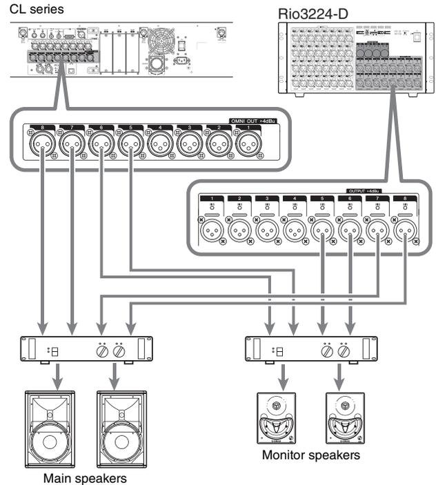
To the OMNI OUT jacks on the CL series and the OUTPUT jacks on the Rio3224-D units, you can patch the output signals from output channels (MIX, MATRIX, STEREO (L/R), MONO (C)), monitor signals (MONITOR OUT L/R/C channels), and the direct out signals of the input channels. For information about patches, refer to “Patching the mixer output to the I/O device” (see page 41) in the Quick Guide section.
