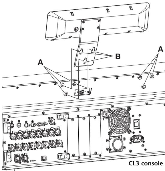
3. Tighten screws 'A' to secure the MBCL, starting with the upper two screws.
