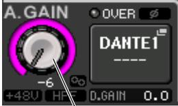
3. Press the +48V button in the GAIN/PATCH popup window as necessary, depending on the microphone you use.
