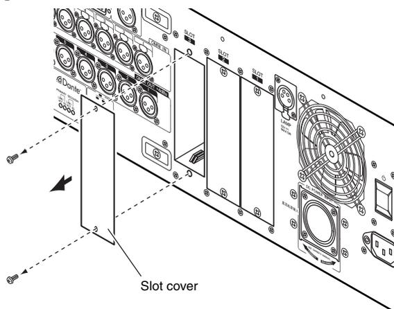
3. Align the edges of the card with the guide rails inside the slot, and insert the card into the slot.
