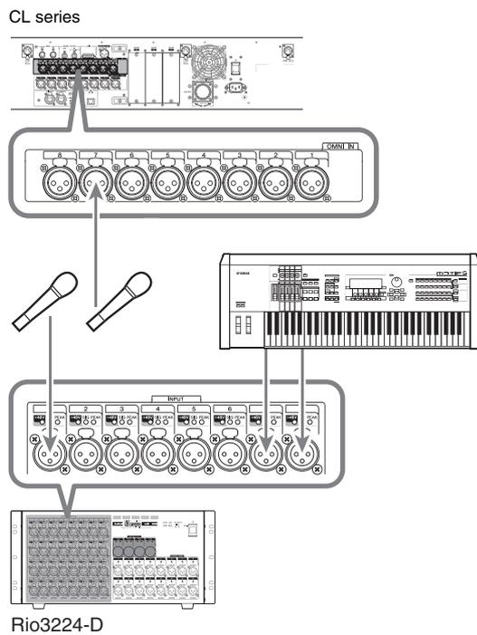
The INPUT jacks on the I/O devices and the OMNI IN jacks are used mainly to connect microphones or monaural line-level devices.
