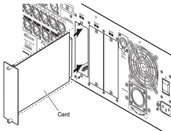
4. Use the screws included with the card to fasten the card in place.
