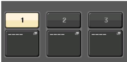
You can also select a channel in the display. Press the button below the desired number to display the CH SELECT screen. First select the tab for a channel group, then select individual channels. To return to the previous screen, press the CLOSE button.
