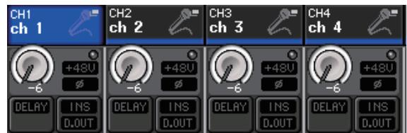
When you press a knob shown in the OVERVIEW screen, a bold frame is displayed around the horizontal row of knobs of the same type. This frame indicates that you can use the multifunction knobs of the Centralogic section to operate the corresponding knobs.
