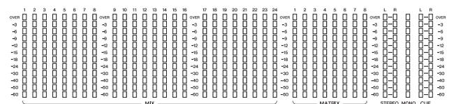
Indicates the level of MIX/MATRIX, STEREO/MONO and CUE channels. You can select the monitoring position from PRE EQ (immediately before EQ), PRE FADER (immediately before the fader), or POST ON (immediately after the [ON] key).
