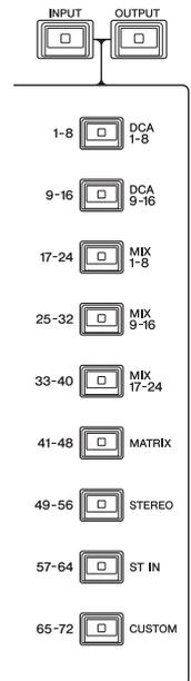
Press the [INPUT] key, then press the key of the channels you want to control.
