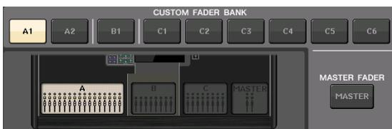
5. In the FADER field, press the channel strip number button.
