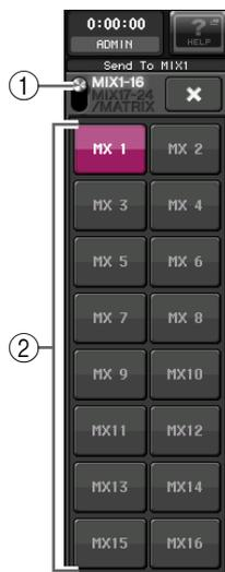
enables you to switch between MIX1–16 and MIX17–24/MATRIX, and the buttons that enable you to select the destination MIX/MATRIX buses.
