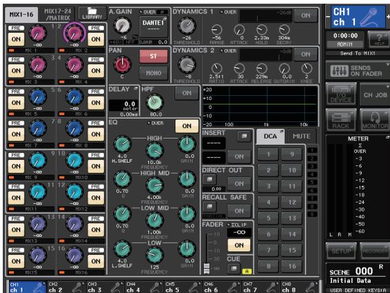
4. Press the [SEL] key of another input channel, and adjust the head amp gain in the same way.
