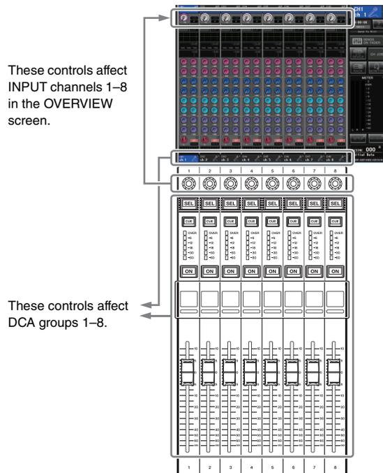
3. To release the channels or DCA groups that were retained for the Centralogic section, press the Bank Select key you operated in step 1 once again, and hold it down until the Bank Select key LED changes from blinking to lit.
