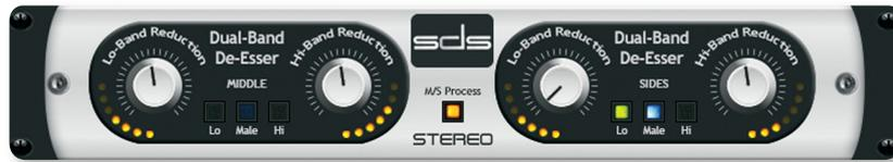
The DE-ESSER is a “must-have” tool for reducing the amount of sibilance in vocal mics while adeptly preserving the natural voice timbre of a performance. Use it to enhance the smoothness of the upper mid to high frequencies in vocals as well as drum overheads and strings, etc. (Inspired by SPL 1239\*)
