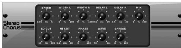
Chorus samples the input, slightly detunes it and mixes it with the original signal to produce a somewhat thicker, shimmering sound. Use it to thicken up background vocals, or to double the sound of brass and woodwind instruments.
