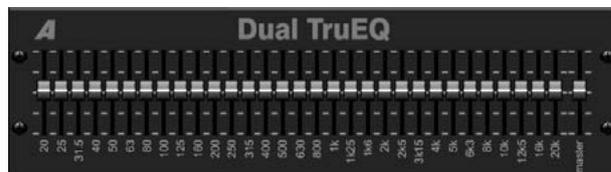
The TruEQ incorporates a special algorithm that compensates for the gain adjustment overlapping effect that adjacent frequency bands have on one another. On a standard EQ, when neighboring bands are boosted together, the resulting effect is magnified beyond what is visible from the positioning of the sliders.
