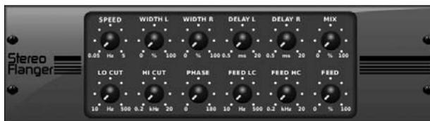
The Flanger emulates the phase-shifting sound (comb-filtering) originally created by applying pressure against the flange of the reel on a tape recorder. This effect creates a unique "wobbly" sound that is quite dramatic when used on vocals and instruments.
