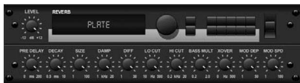
A plate reverb was originally created by sending a signal through a transducer to create vibrations on a plate of sheet metal which were then picked up as an audio signal. Our algorithm simulates that sound with high initial diffusion and a bright colored sound. X32's Plate Reverb will give your tracks the sound heard on countless hit records since the late 1950s. (Inspired by the Lexicon PCM-70)
