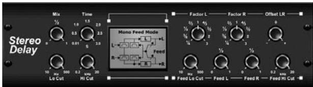
Stereo Delay provides independent control of left and right delay (echo) times and features high and low pass filters for enhanced tone shaping of the delayed signals. Use the Stereo Delay to give your mono signals a wide presence in the stereo field.
