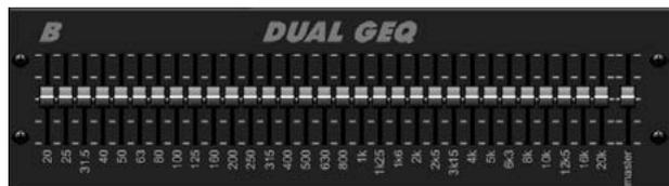
These are standard graphic equalizers that provide 31 bands of adjustment between 20 Hz and 20 kHz. A master volume slider compensates for changes in volume caused by the equalization. A maximum boost or cut of 15 dB is available for each band.
