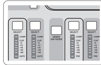
The Sends on Faders function aids with level setting of channels sent to any of the 16 Mix Buses. It is only for channels assigned to Mix Buses 1-16, and does NOT work for DCA groups, main or matrix buses. The Sends on Faders function works in two convenient ways to cover the most obvious situations in a live sound environment :
