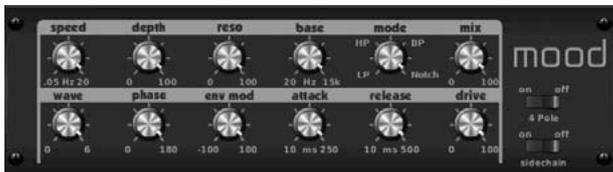
The Mood Filter uses an LFO generator and an auto-envelope generator to control a VCF (voltage-controlled filter), as well as a side chain function where the channel B signal controls the envelope of channel A. When applied to electronic instruments, the Mood Filter can be used to emulate the natural sound of acoustic instruments. (Inspired by the MiniMoog)
