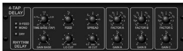
The Rhythm Delay provides 4 stages of delay with independently adjustable gain and rate, allowing unique syncopation to be created in the layered repeats.
