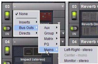
Assigning monitor output to a bus-fed plug-in
