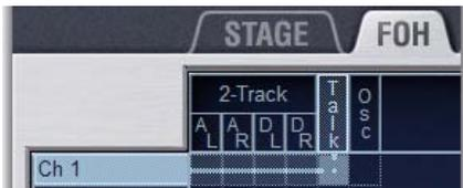
Assigning Talkback input to an Input Channel in the Patchbay
