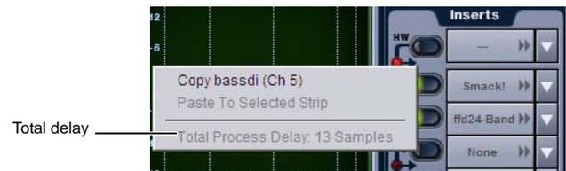
*Viewing cumulative delay by right-clicking the Inserts section*
