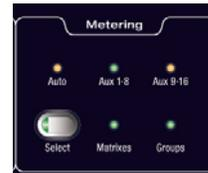
Bus output LEDs and Select switch
