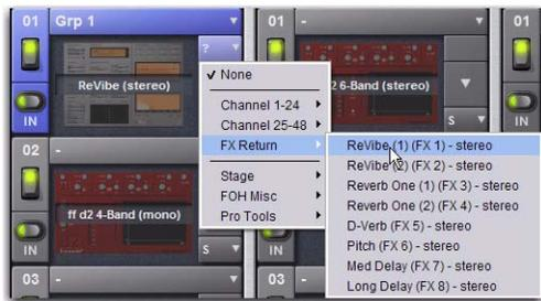
Assigning plug-in output to an FX Return
